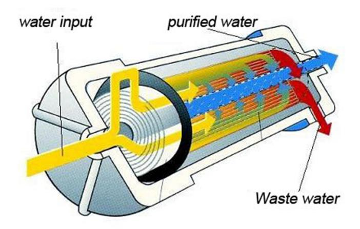
Reverse Osmosis filtration uses a membrane which removes many contaminants from water. It is usually paired with a Granulated Activated Charcoal filter to remove chlorine and many mounts under the sink and have a holding tank. The semipermeable membrane separates many contaminates (which usually have a larger particle size than water) from the water
